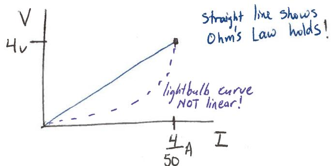
If we swap resistor w/ lightbulb where  $R_{cold} = 7\Omega$ ,  $R_{hot} = 50\Omega$  the resistance is not linear! It is a function of temperature.
