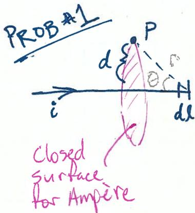
Find magnetic field at P due to current i in wire...
