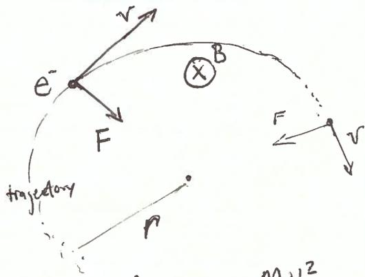
An electron in a magnetic field (into board) moves in orbit like so. Force vector points to center of circle. Speed does not change, force does no work.
