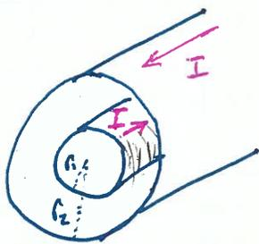
Current I running on inner conductor and returning on outer conductor, find magnetic field everywhere in space
