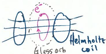
Place glass orbit w/ low pressure gas in field so some electrons can move in a circle
