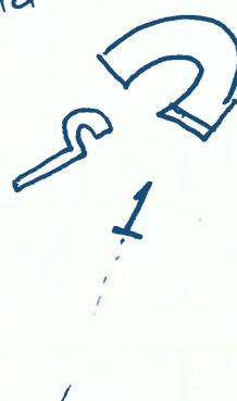
Nail attracted to permanent magnet but when iron wrench introduced the field is altered and nail drops down
