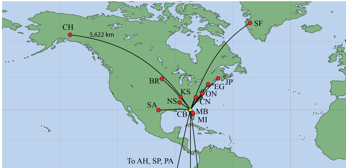
Figure 2-8. Map showing the propagation paths from the ICLRT in Starke, FL to the ELF/VLF receiver stations that were in operation during the 2016 rocket-triggered lightning campaign. The yellow square marks the trigger location.
